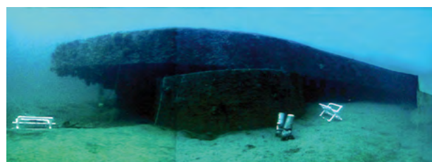
Figure 1: View of the USS Monitor on the seabed at 73 m showing zinc anodes.
