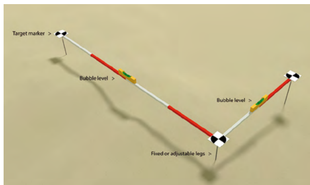
Figure 4. Simple rig to facilitate scaling and orientation of 3D models.
