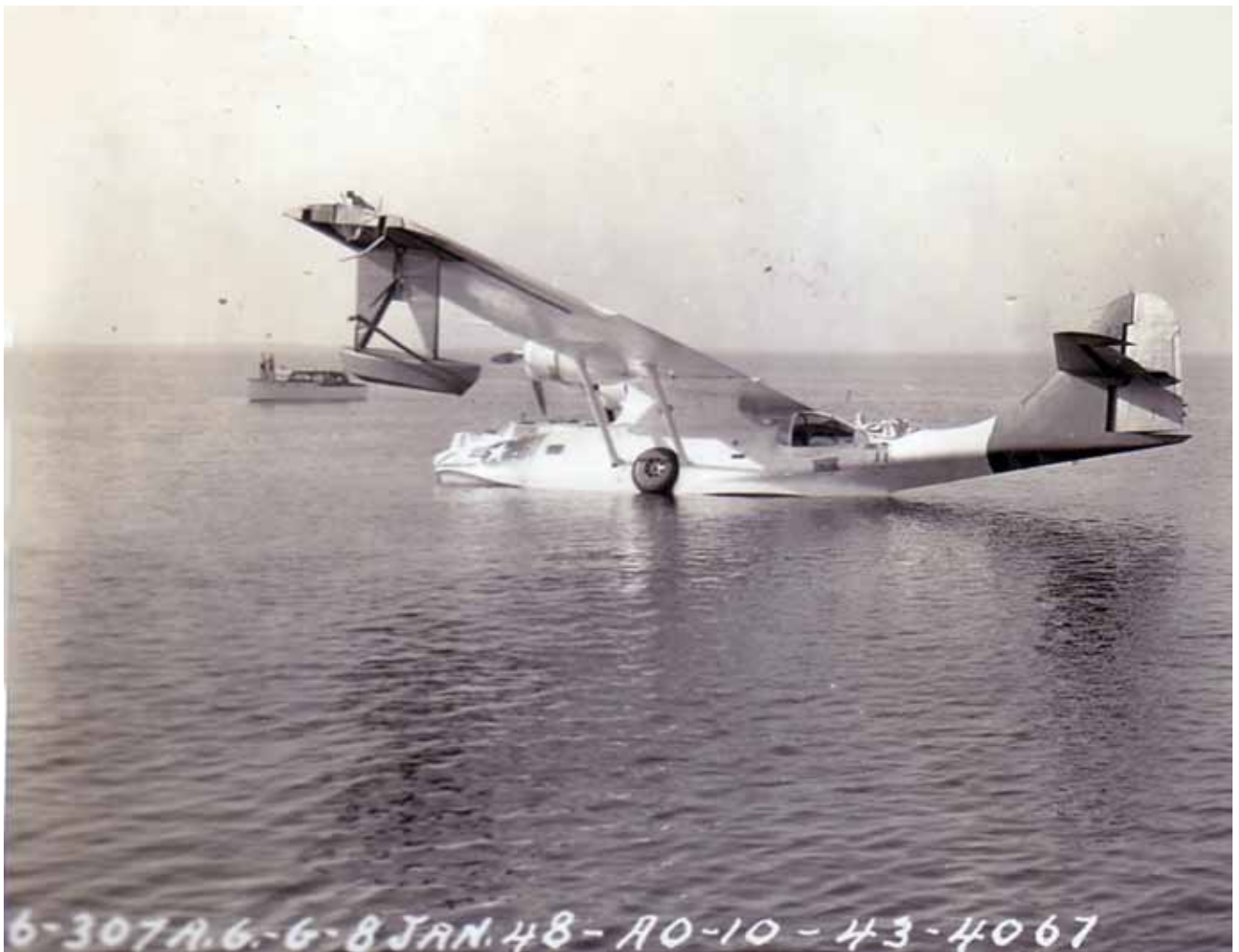
Figure 6. A United States Army Air Force (AO-10) Catalina, which suffered pontoon damage after a heaving landing in Tampa Bay, Florida. It is actually Serial # 44-34067 not 43-4067, which was a B-25J that crashed in Switzerland on 7 February 1945. This Catalina was later salvaged—it did not sink' (Ragnarsson 2006; Johnson 2003). Note: the Catalina almost capsizing to starboard due to the submerged starboard wing tip and pontoon. Both pontoons have been damaged.
