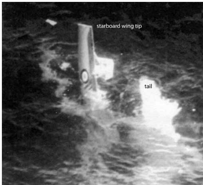
Figure 7. 'NZ4046 — the final moments before sinking' (Harrison, et al. 1997: 231). Note: although this Catalina did not burn, it is capsizing given that the starboard wing, seen here, is dragged down by the fuselage and port wing.
