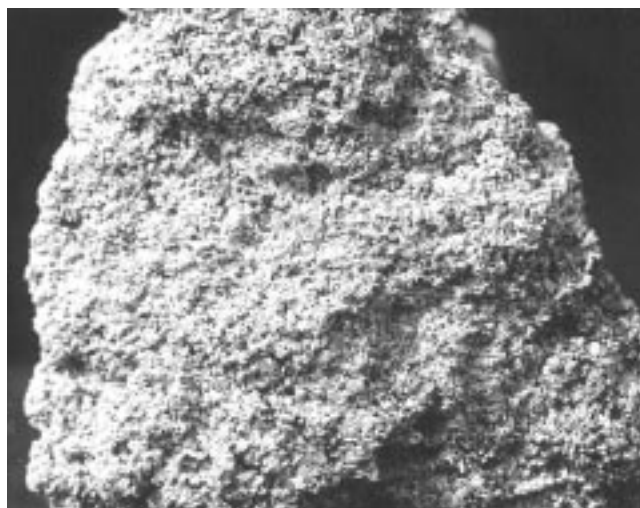
Figure 8. Calcarenite (limestone) dripstone material from Barbados. The sharp skeletal texture of the raw stone is very evident. Photo: A.R.D. Porter.
