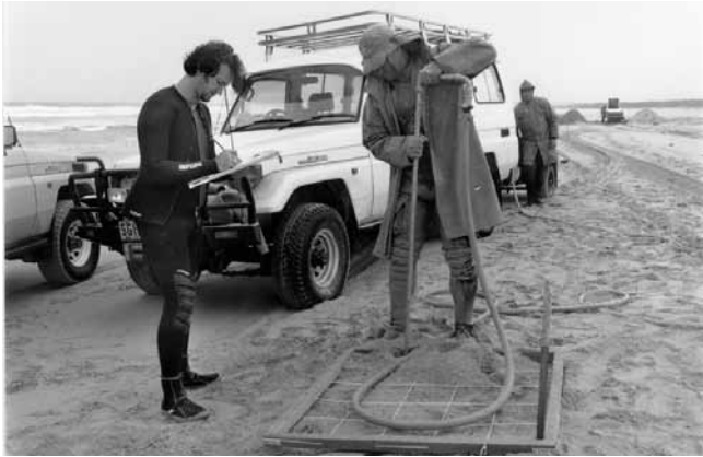
Figure 8. A compressed air probe accurately placed the corners of the caisson in relation to the iron object. (Photo: S. Humphries)
