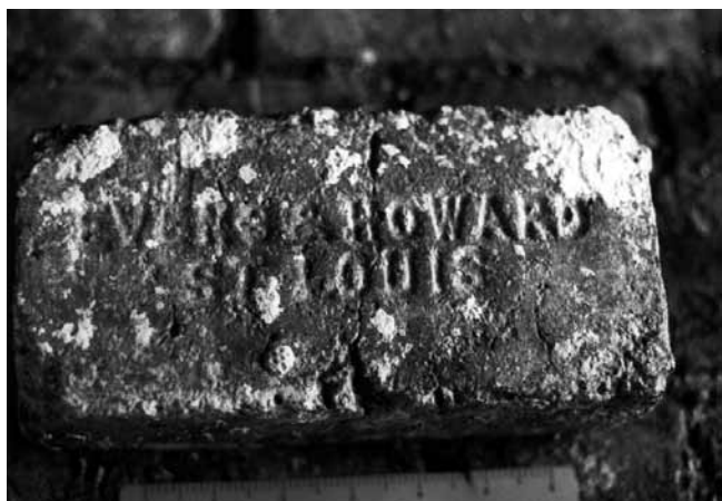
Figure 5. Yellow firebrick from Bird Key Wreck, showing markings, 'EVENS & HOWARD, ST. LOUIS'.
