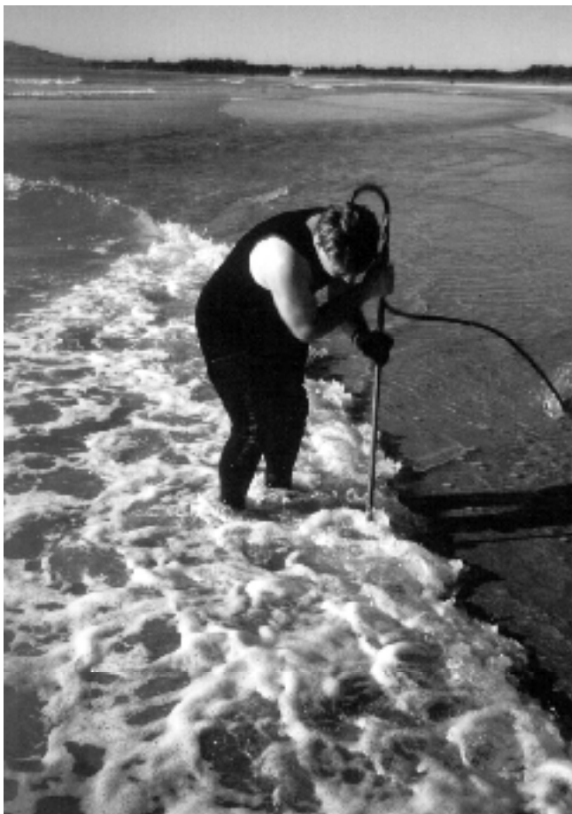
Figure 4. Colin Brown (MHL) sinking the 3 m water probe forward of the engine area of the steamer Emu .
