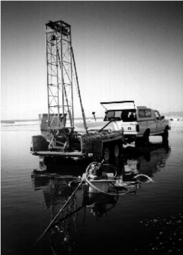
Figure 1. View of box trailer with reservoir and gantry for retrieval of the 6 m water probe. The 3 m water probe and pump are visible in the foreground.
