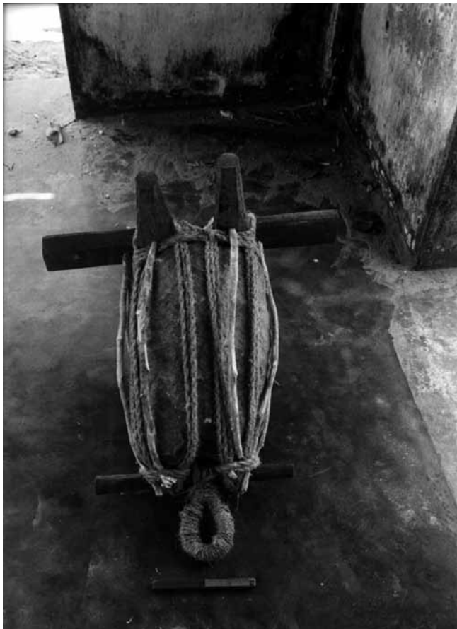
Figure 6a. Double-stocked mooring killick at Kathaluwa-Ahangama, Galle District, Sri Lanka (photo: Kapitän).
