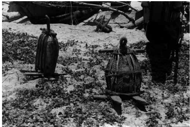
Figure 6b. Double-stocked mooring killicks at Kathaluwa-Ahangama, Galle District, Sri Lanka (photo: Kapitän).
