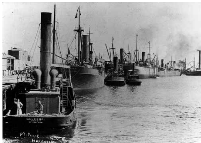
Figure 2. The Nelcebee at the Port Pirie wharf, the presence of the ship Baldersby dating the photograph between 1913 and 1918. Clearly to be seen is the iron house extending back from the saloon—the pump room (ex-galley) and the present engine room trunk are remnants—and the widened base to the house in the area adjacent to the boiler which was later converted to form an after hatchway. Also visible is the lifeboat carried on the port side, and the towing hook mounted on top of the house. SAMM:7365.
