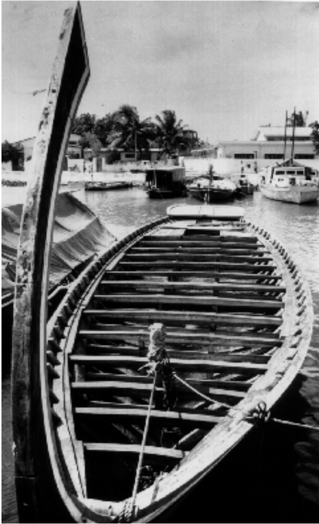
Figure 2. Dhoni without deck planking showing the many thwart beams.
