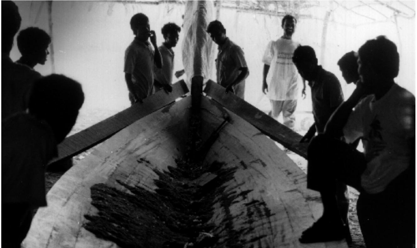
Figure 6. Plank being held in place to determine the shaping that is needed.
